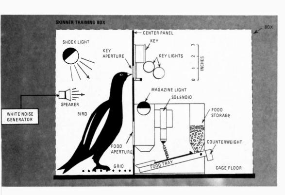
Fig. 2. Typical Skinner training box. Feeding and cueing mechanism are housed in one side of the box while the bird lives on the other side. White noise masks out environmental disturbences. Lights are used in various ways to give cues.
