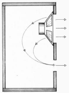
The size of the vent is important, for it is a combination of this and the physical dimensions of the enclosure, that determines the behaviour of the system and provides the smooth, extended low frequency response for which this type of enclosure is renowned.
