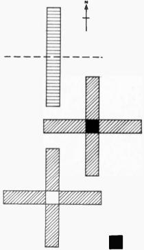
Mills of Sydney University this antenna provides a very narrow pencil beam and can resolve very fine details of any noise source being studied. A combination of techniques is used to enable the beam to be aimed almost anywhere in the sky. The East-West arm is fully steerable in altitude while the North-South arm uses a lobe phase-switching technique.
