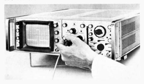
In the new Model 180C/D version of its 180-series Oscilloscopes, Hewlett-Packard has increased trace brightness by a factor of about five, giving a writing speed of 1500 cm/ $\mu$ s. (Standard P31 phosphor as photographed with 10,000 ASA film, fl.3 lens. 1:0.5 object-to-image ratio without film fogging. Substantial increase in writing rate can be had with P11 phosphor, faster lenses, and use of film fogging techniques.)
