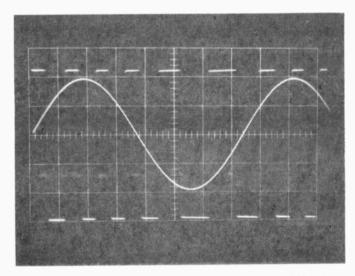
Fig. 1. (a) Square wave signal to record head of Electrodata FM 300. (b) Sine wave input
