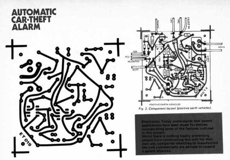
Fig. 1. Foil pattern of printed circuit board, reproduced full size.
