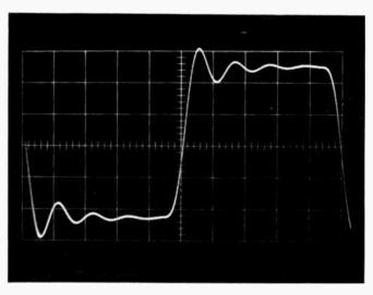
Fig. 4, Record/Replay Response of Bruel & Kjeer 7001 to 200Hz square wave.
