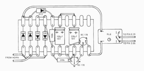
Fig. 7. Constructional details of circuit shown in Fig. 6.
