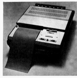
The new Schlumberger/SIS optical UV recorder model OM 4501 allows the simultaneous recording from one to eight parameters in cartesian coordinates. The traces are recorded on daylight printing paper, sensitive to ultra-violet rays and are chemically developed following exposure to daylight.
