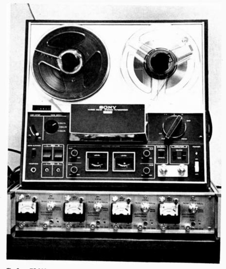
The Sony TC 366 tape deck is fitted with a four-channel head,
