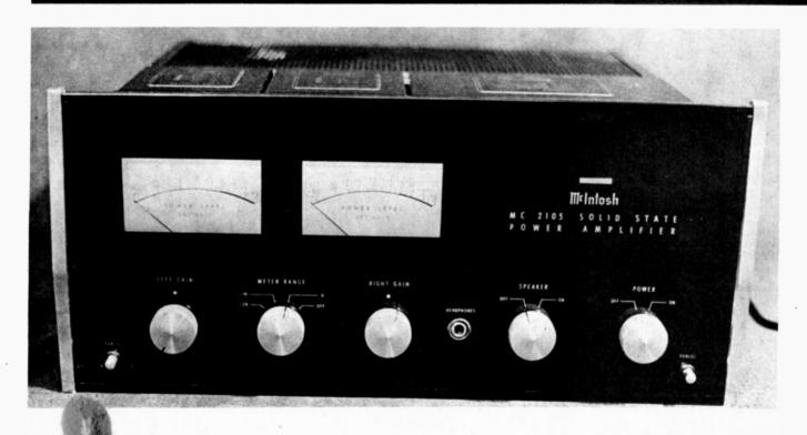
THE motosh MC2105 solid state power amplifier is very similar in appearance to the preamplifier. The external finish is identical, with a black glass front panel with chromed trims at each end and machined aluminium knobs.
