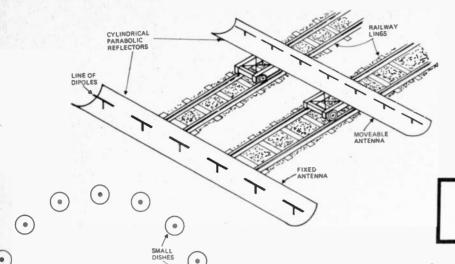
Fig. 18. Aperture synthesis antenna used at Cambridge (UK).
