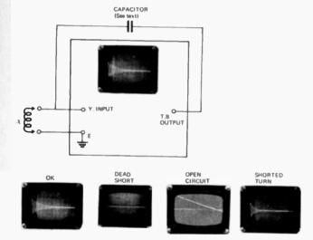
Transformers and inductors can be checked for open circuits, short circuits, shorted turns, etc., by this very simple method.
