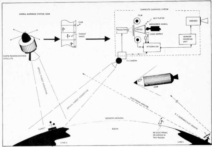
Fig. 1. Proposed animal-guidance system for ICBM. Initial target data is acquired by photoreconnaissance satellite. System operates with superimposed images and can't be jammed.
