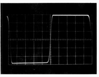
Fig. 3. Record/Replay Response of Electrodata FM 300 to 200Hz square wave.
