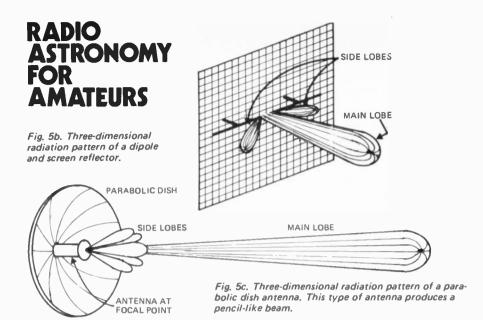
as a fraction of the physical area of the antenna being considered. The value varies between 0.5 and 0.9. It is dependent on the direction of arrival of the wavefront, being at a maximum along the axis of the main lobe.
