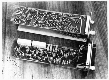
BOTTOM: Electrodata record module - TOP: Replay module.
