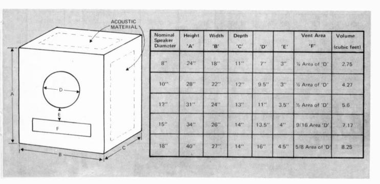
Table I — this table and the associated drawing shows how to design a reflex cabinet if no data other than speaker diameter is known.
